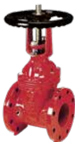
Series 45/56 Flanged gate valve with rising stem OS&Y DN50-300: 17.2 bar (250 PSI) DN350-400: 13.7 bar (200 PSI) PN16 drilling Ductile iron UL/ULC listed, FM approved
