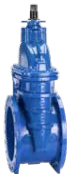
Series 55 Flanged gate valve with wrench nut NRS DN450-600 13.7 bar (200 PSI) PN16 drilling 316 stem Ductile iron UL/ULC listed, FM approved
