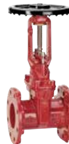
Series 145/46 Flanged gate valve with rising stem OS&Y DN50-200 17.2 bar (250 PSI) ANSI drilling class 150 Ductile iron UL/ULC listed, FM approved
